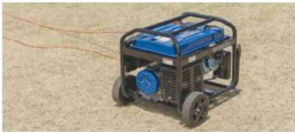
SAFETY FIRST: Make sure your generator is ventilated and operated in open areas to prevent carbon monoxide build-up
